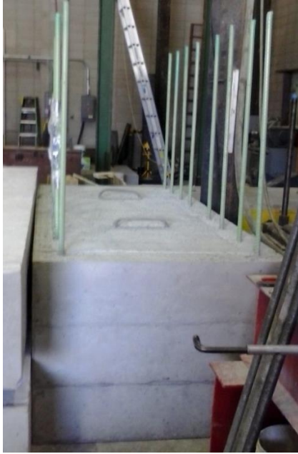
Figure 20. CIP pile cap
