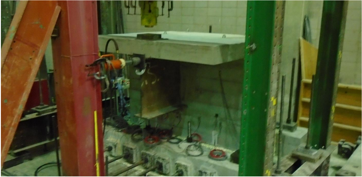
Figure 56. Laboratory loading, horizontal and vertical actuators
