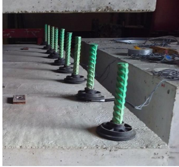
Figure 31. Neoprene disk, seal plug and shim
