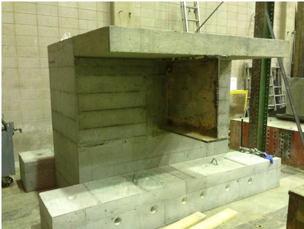
Figure 22. CIP integral abutment specimen
