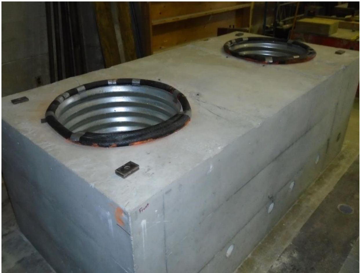
Figure 48. Pile cap with backer rod seal
