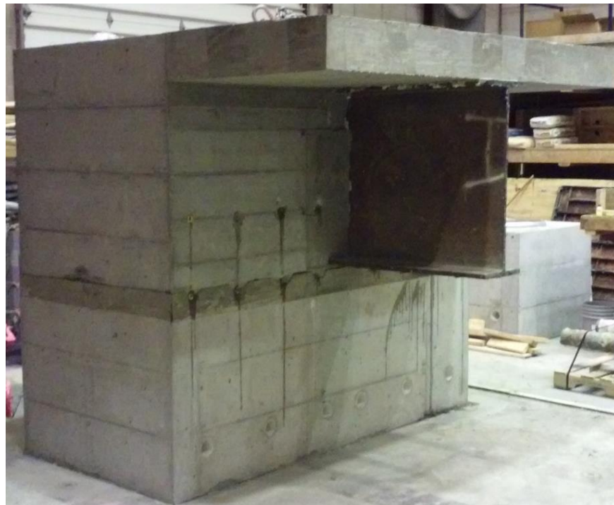
Figure 35. Completed grout bed and coupler grouting
