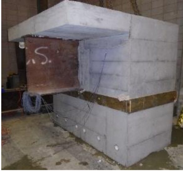
Figure 49. Grout bed formwork back
