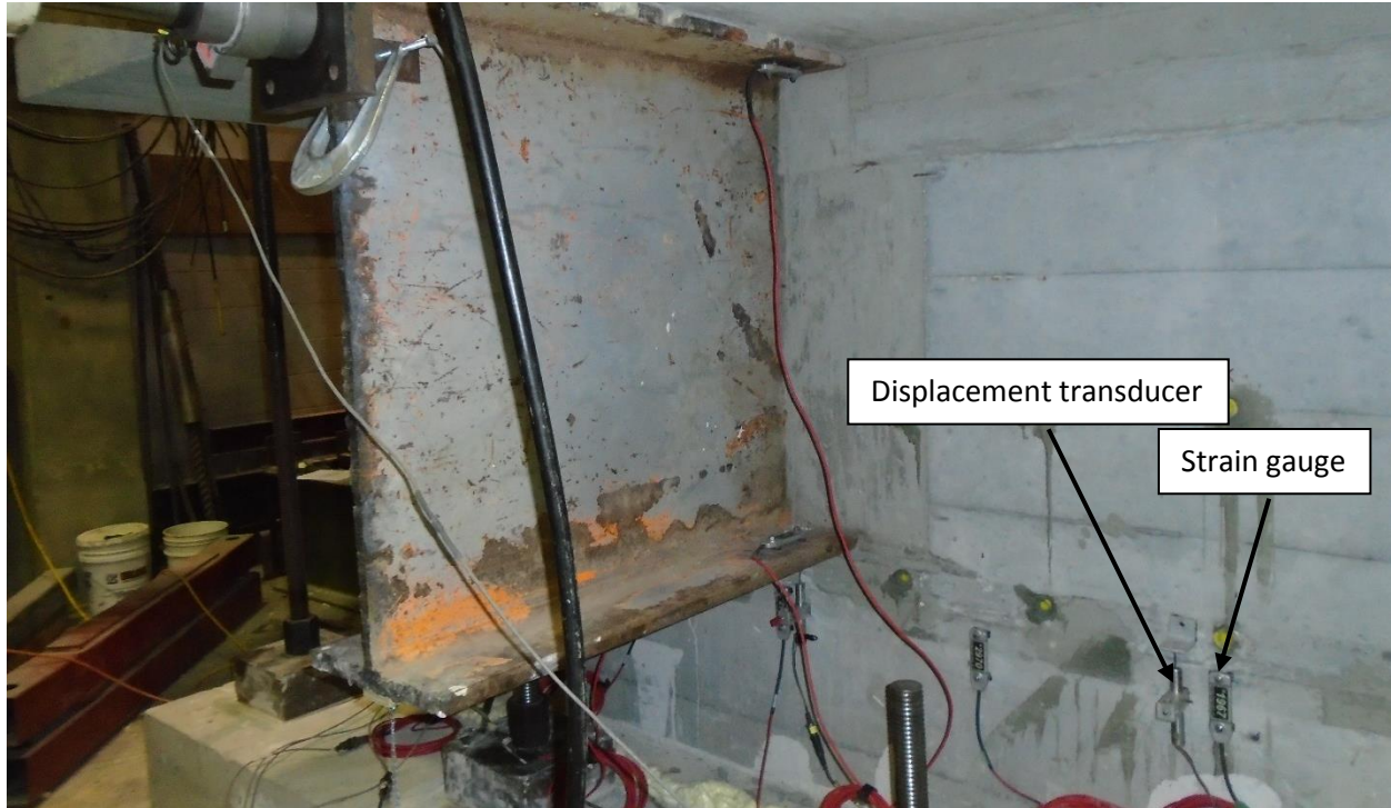
Figure 63. Front face of the abutment during horizontal loading
