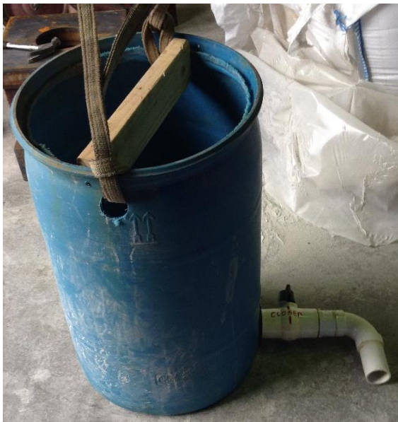
Figure 51. Grout funnel system
