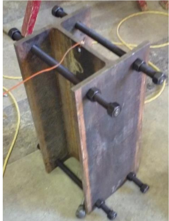
Figure 42. HP section with threaded rods
